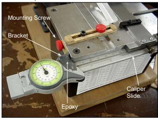
After removing the plastic jaws, a brass bracket was affixed to the caliper dial housing with some epoxy. Merritt's first efforts at gluing the bracket didn't meet with much success. After several adjustments, the assembly fell apart. So it was back to Ace where a product called CP-7 was purchased. As of meeting time, the stuff was still holding firm.
